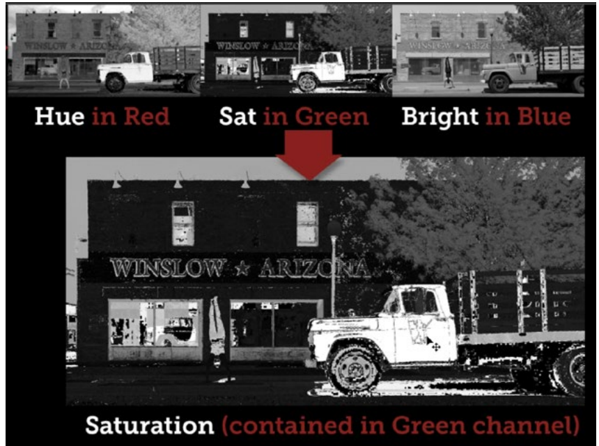
After running the HSB filter, the Saturation information is being stored in the Green channel, and here we are viewing that channel in the Channels panel. The most colorful areas are white and the least colorful areas are black.
