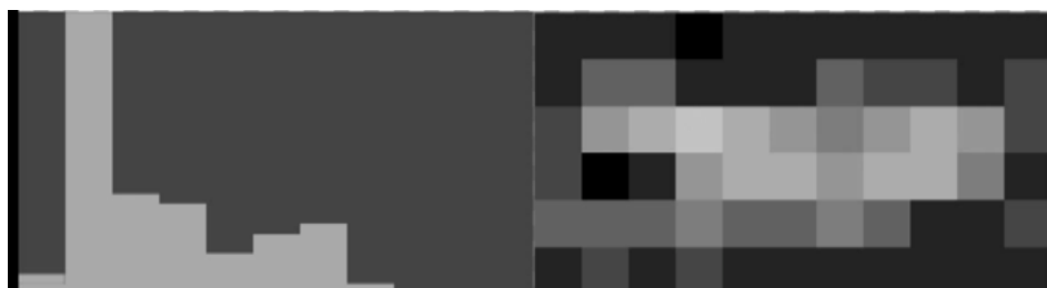
Here we have our oversimplified version of the image (to 11 brightness levels) along with the resulting histogram chart.
